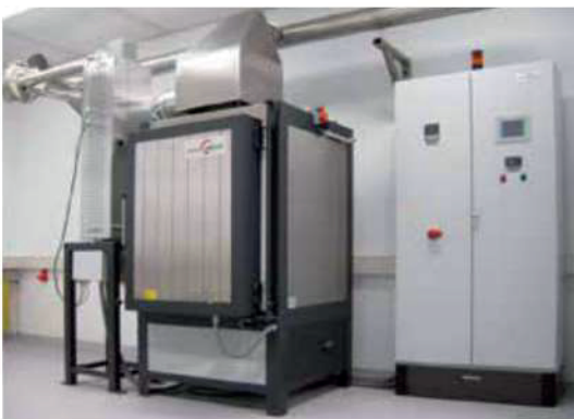
Chamber furnace up to 1400 °C for de-binding and sintering in one process, with catalytic waste gas purification system
